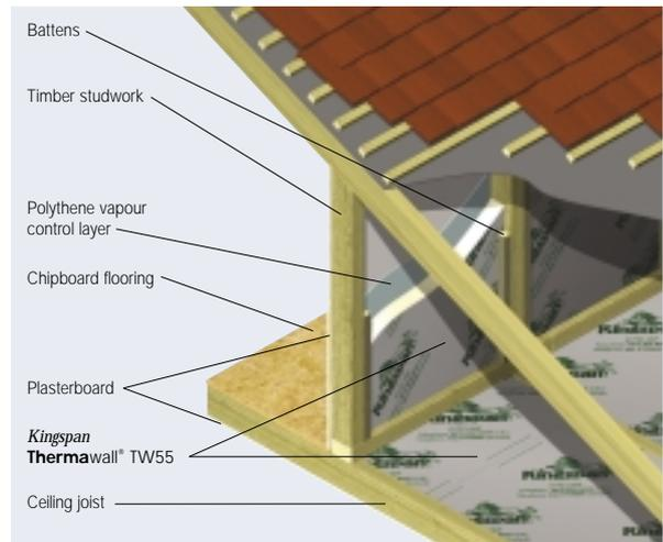
Figure 4 Dwarf Wall – Insulation Between Studs
